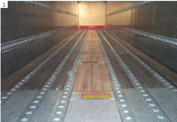
N. 3 - 6 Vie a rulli con rulli motorizzati 6 Roller tracks with powered rollers
