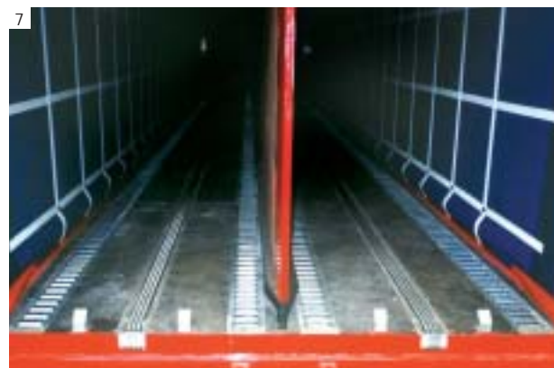
N. 7 - Sistema standard 4 vie a rulli e 2 catene con stop-pallet Standard 4 roller tracks and two slipchains system with pallet-stops
