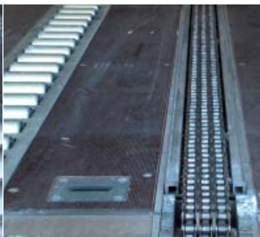
Rulli e catene per movimentazione pallets di legno Vehicle-mounted slipchain systems for loading and unloading of palletised goods
