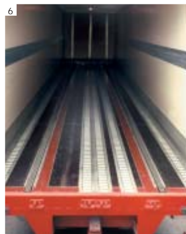
N. 6 5 Vie a rulli e due catene 5 Roller track and 2 slipchain system
